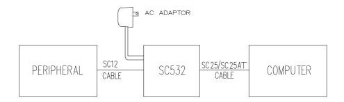
Figure 2 Connection Block Diagram
